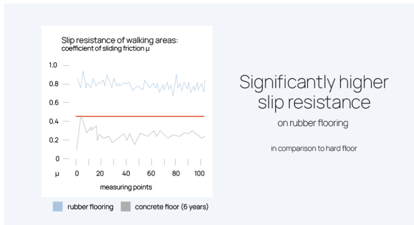
DGL testing of walking area flooring, Source: Reubold, 2004
