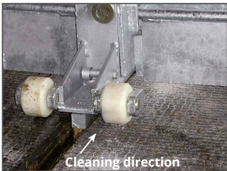
Center bracket rests on wide plastic rolls
