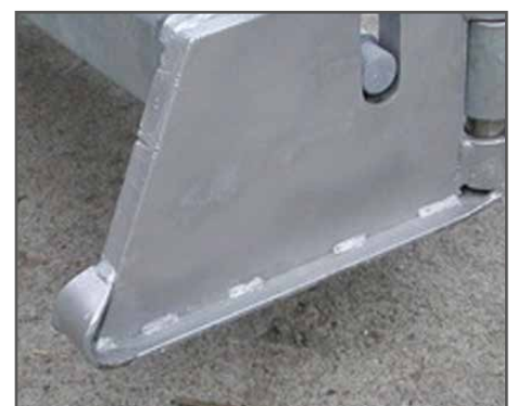
Wide and bent up side skids
