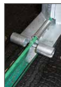
wide bearing for center bracket, welded on rod iron
