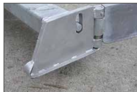
wide and bent up side skids
