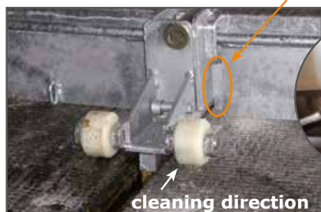
center bracket rests on wide plastic rollers
