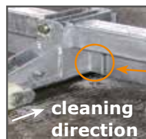
cleaning flap back stop: no contact to the surface
