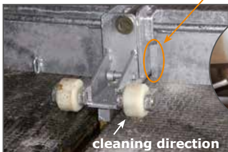
center bracket rests on wide plastic rollers
