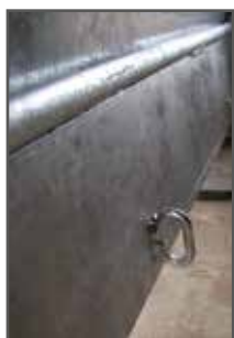
chain links welded on
