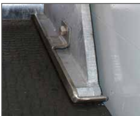
wide and bent up side skids, screwed on
