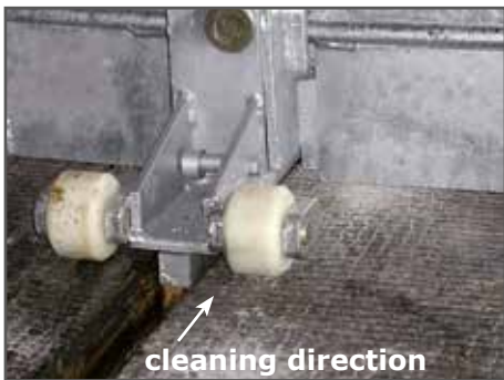
center bracket rests on wide plastic rolls
