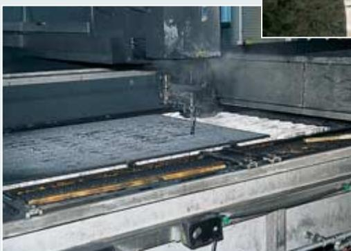
*The shape of each individual slot is recorded, marked and entered into the computer. Then the slots are cut by a waterjet cutter.*
