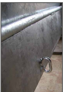
Chain links welded on
