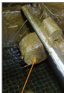
Cam block on main cleaning flap
