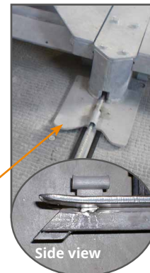
Wide bearing for center bracket, welded on round bar
